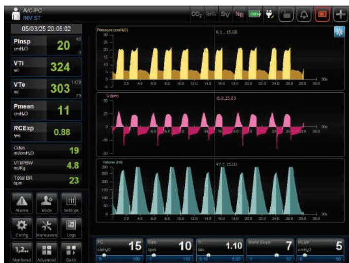
Figure 3. Airflows obstruction with spontaneous breathing and Smart Trigger activated. Note no missed triggers and many of the breaths were triggered by negative flow (White). Smart Trigger showing the improvement of assisted ventilation when compared to pressure/flow triggers.
