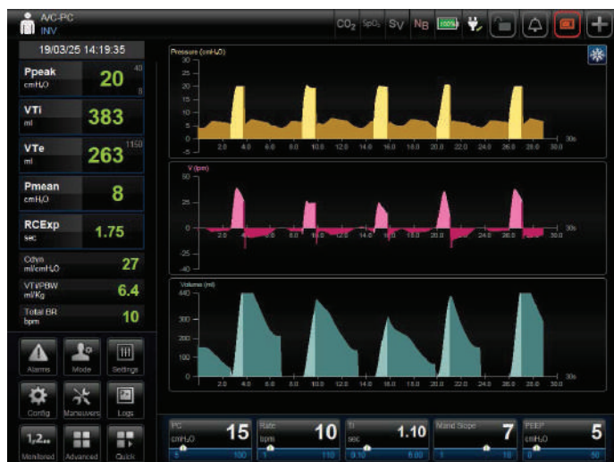
Figure 2. Assisted ventilation with pressure/flow triggers. Airflow obstruction with spontaneous breathing with a tandem trigger setting of flow and pressure. Note the mis-triggers (White) and the pressure drop (Red) required to trigger the ventilator.
