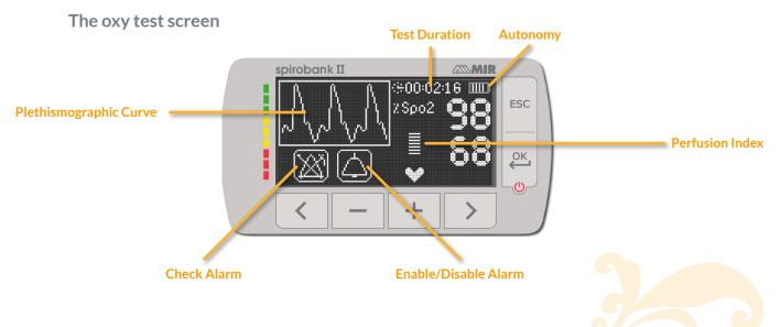
When done with the oxy test **press the ESC button** to end test and see results on the screen.
